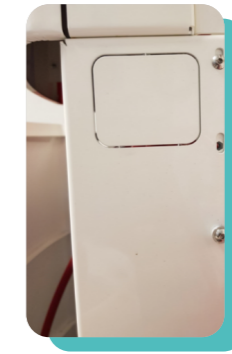
Opercul : passage tuyaux raccordement
